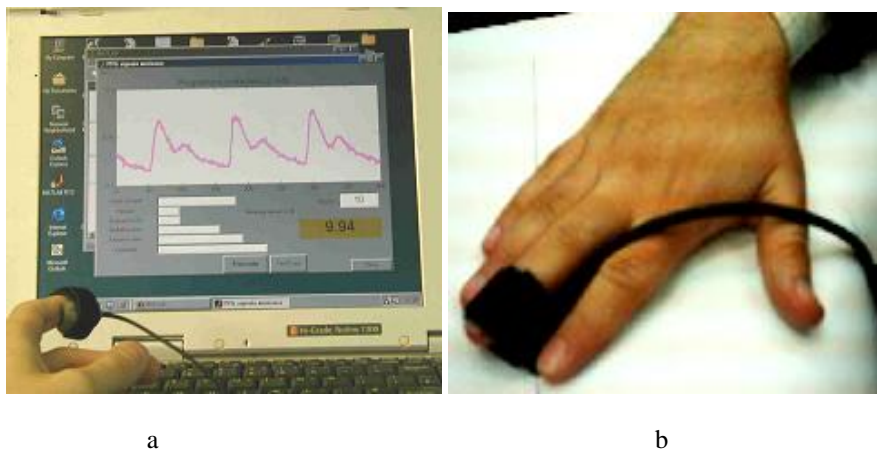
Fig.4. The PPG contact probe (a) and its application for the fingertip monitoring (b)
