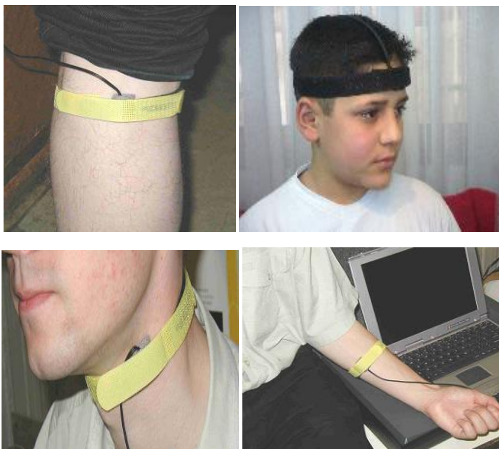
Fig. 5. Application of the PPG contact probe at forehead, neck, forearm and knee
