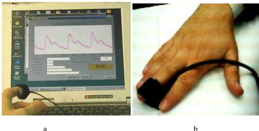
**Fig.4.** The PPG contact probe (a) and its application for the fingertip monitoring (b)
